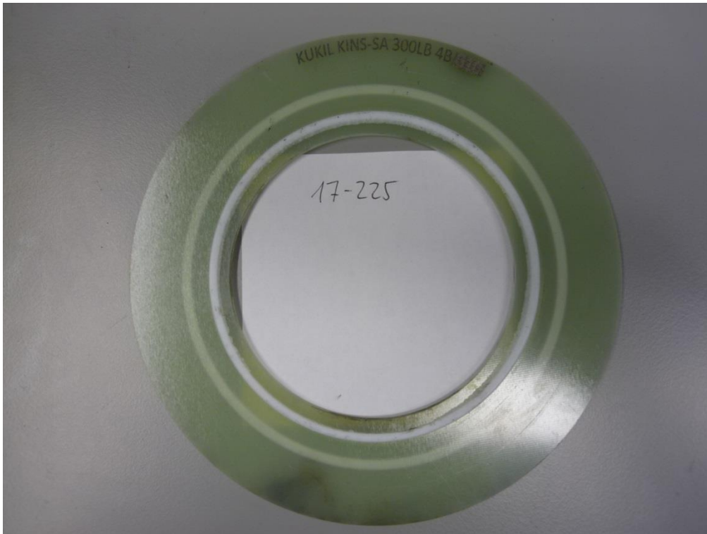
Shell electrical isolation test according MESC SPE 85/300 - 3.3.15 Insulation Gasket K/# KINS-SA (after test)
