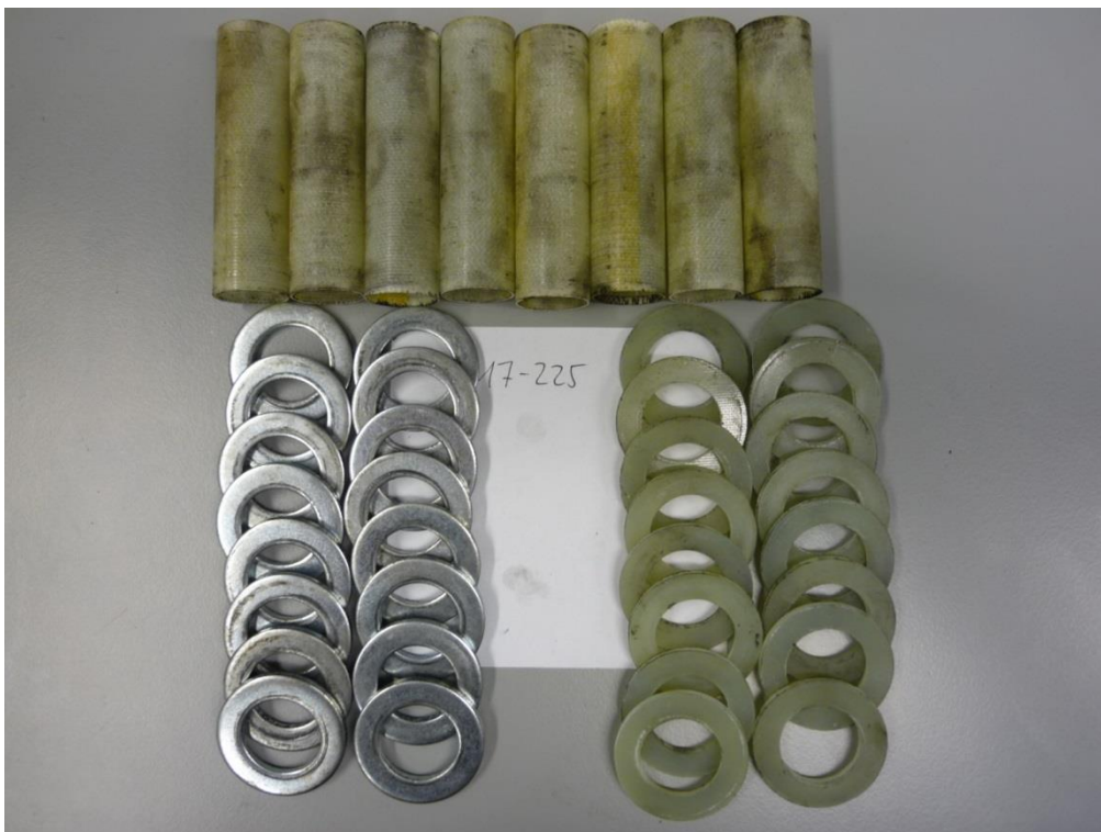
Shell electrical isolation test according MESC SPE 85/300 - 3.3.15 Insulation Gasket K/# KINS-SA (insulation gasket kit)
